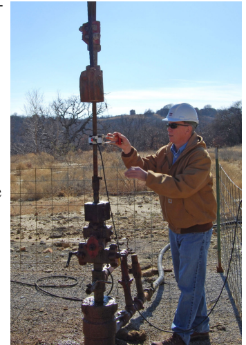
Installing Quick Clamp on rod string
