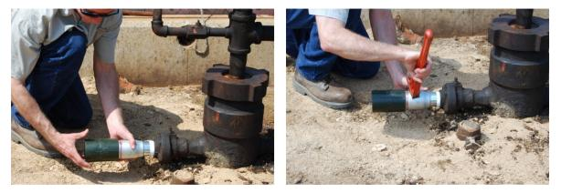
2. Hand-fit the gun to the adapter. Finish tightening the gun with the provided spanner wrench, which fits into the notches on the base of the gun body. Proceed with the fluid level test.
