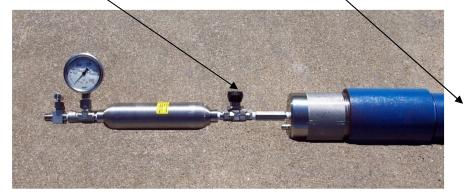
4. Fill expansion chamber with wellbore pressure. The gauge will register pressure. Close the **ball valve** to seal off the expansion chamber from the wellbore.
