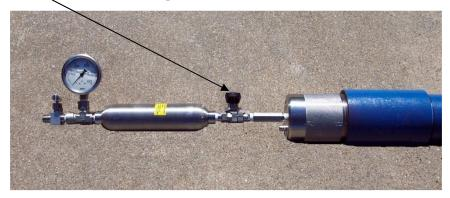
5. Use the **needle valve** (the valve closest to the gauge) to bleed down the pressure in the expansion chamber to below wellbore pressure by watching gauge. Close the needle valve once the correct pressure is reached.
