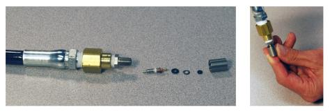
With the gun maintenance tool, unscrew the internal valve core from the end of the charge hose, and replace it with a new valve core. Hand tighten securely. Then, rebuild the charge hose tip, as shown above, first placing the small o-ring in the bottom of the tip, followed by the flatwasher and then the larger o-ring. Insert the end of the charge hose into the tip and hand tighten securely.
