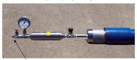
3. Slowly open the **needle valve** to remove all pressure from the gun.
