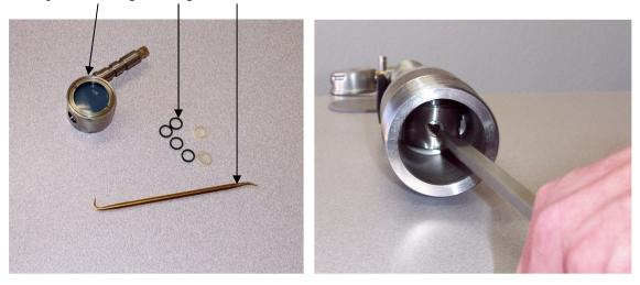
To disassemble the gun for maintenance, first remove the **internal microphone by** removing the microphone retainer bolt from the bottom of the gun, using a flathead screwdriver or your maintenance tool, as shown above right.
