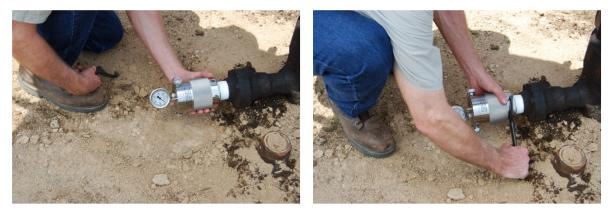
2. Open the backside casing valve, shown below left. This will allow the compressed gas shot to travel down the wellbore to find the fluid. Next, close the casing flow line valve, shown below right. This prevents the compressed gas shot from going down the flow line instead of down the wellbore.
