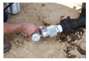
4. To charge up the gun, first make sure the pressure bleed knob is turned closed. Open the valve on the compressed gas bottle. Press the stab-in connector on the charge hose into the "Fill" connection on the gun. Note: When the charge hose stabs into the fill valve, some gas will blow back from the insertion point. This is normal, and helps keep the charge area free of debris.
