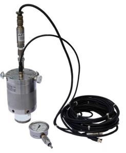
afterflow in the wellbore directly before the shot. The quickconnect on top of the Pressure Pulse Gun -- both 1,500 and 3,000 psi -- allows for easy connection of a same-rated 1,500 or 3,000 psi pressure transducer in place of a gauge.
