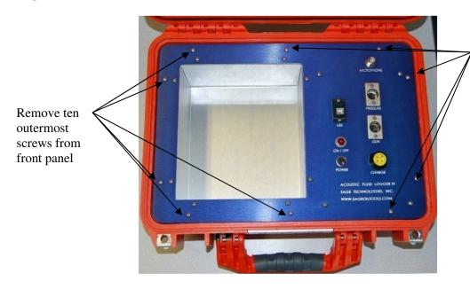
Remove ten outermost screws from front panel
