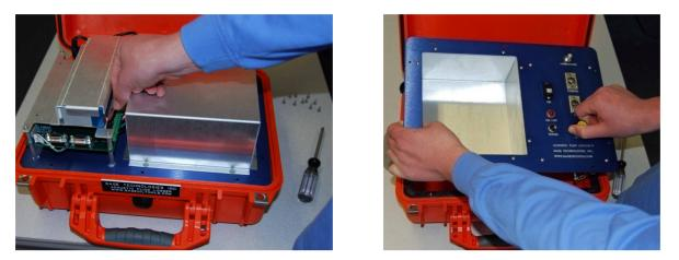
Reconnect the battery; be SURE to connect the red battery connection wire to the red battery pole, and the yellow connection wire to the black battery pole. **Important: At this point, lift the front panel and clean out any dirt or debris that has fallen inside the orange box. Any stray screws, metal parts, paper clips or excessive dirt may harm the circuit board.**
