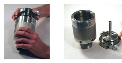
Remove the Shuttle Valve assembly by using the two 3/8" Allen wrenches, as shown below. Pull the shuttle valve out of the bonnet.
