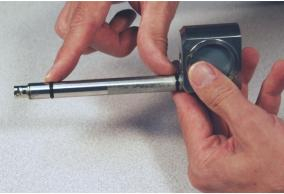
For maintenance on the fill valve, remove it with the thick, notched end of the gun maintenance tool, turning counter clockwise. An o-ring and the valve core will be exposed under the fill valve. Remove the valve core with the tapered, notched end of the gun maintenance tool, turning counterclockwise. Replace the old valve core with a new one, and hand tighten, using the maintenance tool. Replace the o-ring, if necessary. Replace the fill valve and tighten securely.
