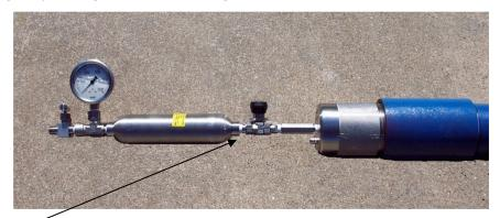
2. Open the **ball valve** to connect all pressure passages in the gun.
