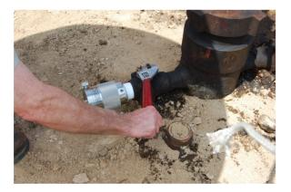
13. Use the spanner wrench to loosen the gun from the wellhead. Once loosened, the gun may be rotated and removed by hand. After the gun is removed from the wellhead, remember to open the casing flowline valve. Repack the gun and accessories into the black case for easy transport from the well site.
