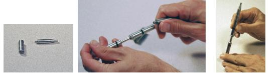
When replacing any of the o-rings, clean the shuttle valve passage and grease the shuttle valve orings with silicone lubricant. Reinstall the shuttle valve with the long end of the shuttle valve to the "Fire" side of the gas gun.
