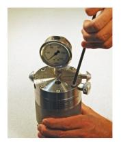
After removing the eight screws from the top, separate the bonnet top from the gun body for maintenance. Replace and grease the large O-ring on the gun bonnet top, as shown below right, with silicone lubricant. Reassemble the top, applying copper anti-seize to each of the socket-cap screws, and again tightening opposing screws on the bonnet top to avoid o-ring damage.
