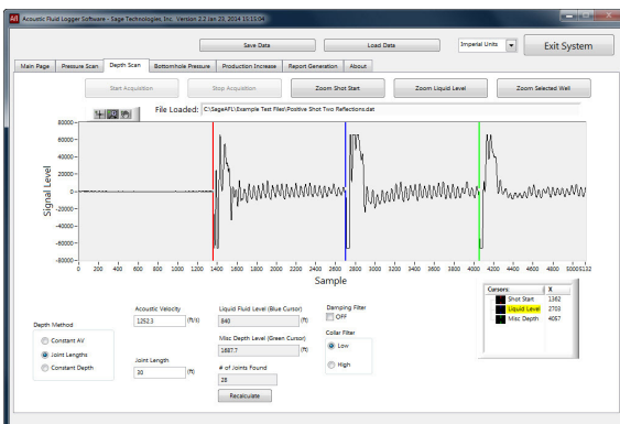
Sample Fluid Level shows compressed gas shot (red line), fluid level (blue), and second reflection of fluid (green).
