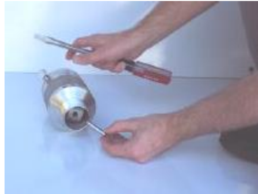
Photo 3, Remove retainer bolt
