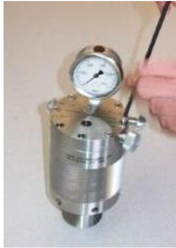
Photo 4, Loosen screws on top of gun
