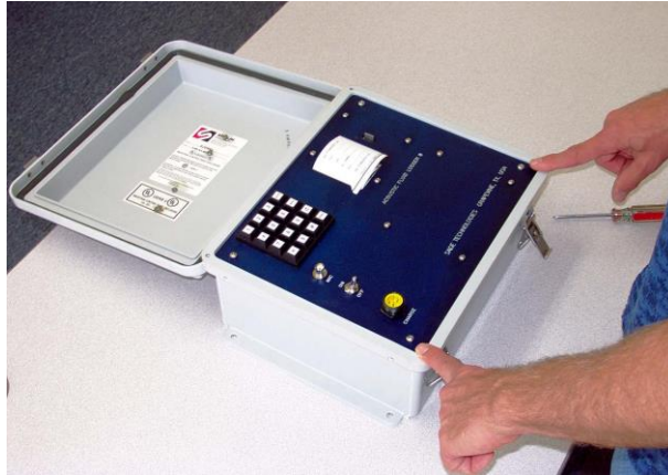
Photo 1, Remove front panel from Acoustic Fluid Logger
