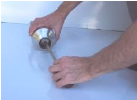
Photo 2, Loosen retainer bolt
