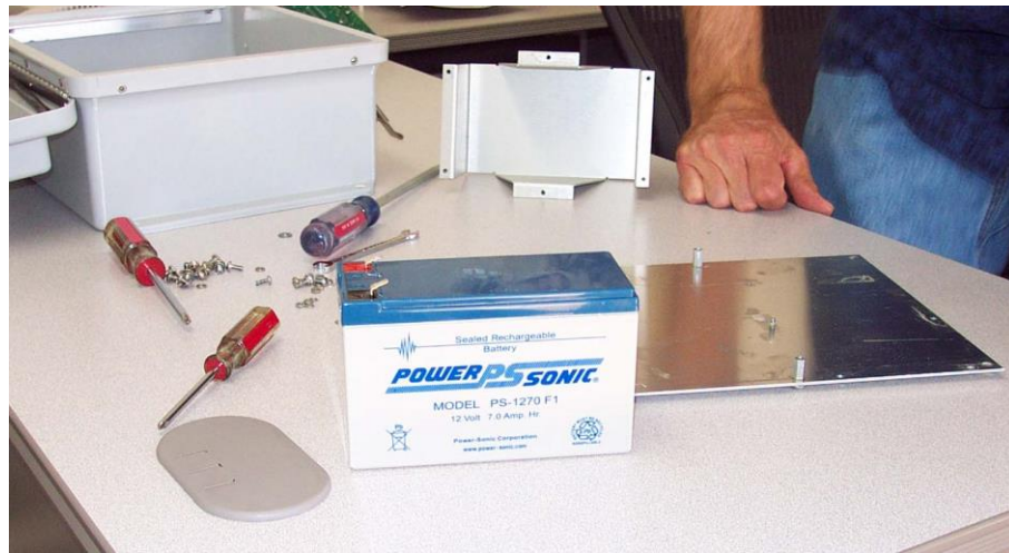
Photo 9, Replace with standard motorcycle battery, 12-volt, 7.0 amp
