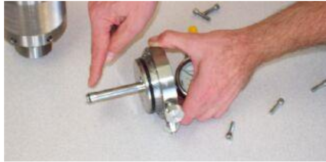
Photo 7, Replace small black O-ring on blast stem
