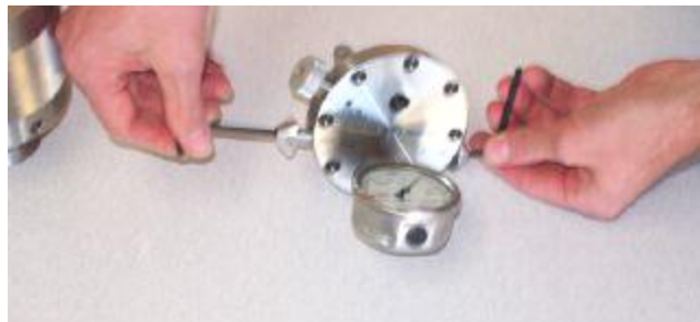
Photo 8, Remove shuttle valve with two Allen wrenches
