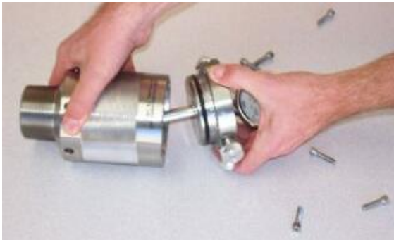
Photo 5, Separate top and bottom of gun
