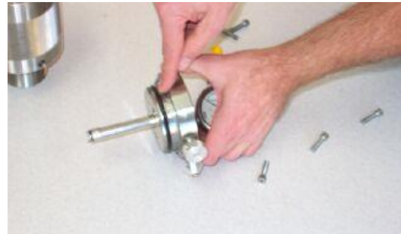
Photo 6, Replace large black O-ring on gun top
