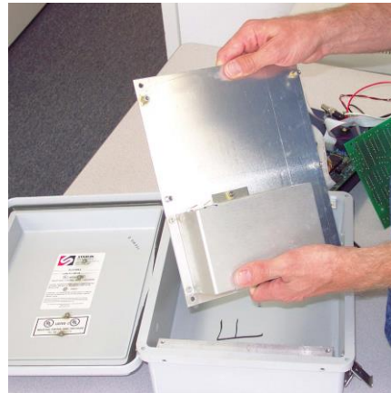
Photo 7, Remove battery plate from box
