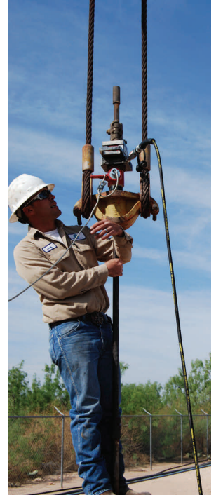
Horseshoe Load Cell in operation with String Transducer
